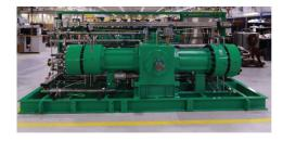
Lastly, Sundyne's PPI diaphragm compressors have been used to compress hydrogen from electrolyzers into storage tanks. Hydrogen is essential to all SAF & RD production pathways. Sundyne's diaphragm compressor is highly reliable, leak-free and guarantees that the hydrogen is not contaminated. It offers superior Mean Time Between Maintenance due to longer life diaphragms.
