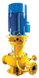
(EPCs) that service these refineries, a unique combination of materials has been created specifically for HF acid service. This industry approved design features Alloy C276 wrought parts and Alloy C22 castings. The pump casing casting uses a specially adapted and repeatable manufacturing process that ensures integrity in HF acid service.
